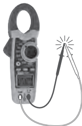
Continuity Measurement: Buzzer Sounds
