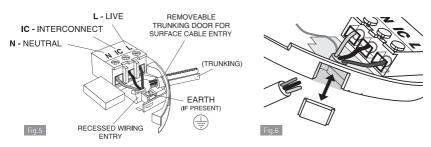
**4.** If the mains wires are recessed, bring the wires through the rear hole in the mounting plate as shown in Figure 5.
