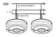
Make electrical connections as shown in Figure 9. Wiring must be installed in compliance with local regulations.
