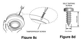
PUSH UP CATCH & TWIST ALARM ANTI-CLOCKWISE TO REMOVE
