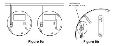
A maximum of 250 metres of two core, 0.5mm<sup>2</sup> to 0.75mm<sup>2</sup>, stranded signal cable can be used, (maximum resistance between detectors 50 ohm). The Alarms are interconnected by wiring all the terminals marked 1 together, and all the terminals marked 2 together (see in Figure 9a). Note: Draughts from wiring openings, conduit, or mounting boxes/holes, may blow smoke away from the sensing chamber,
